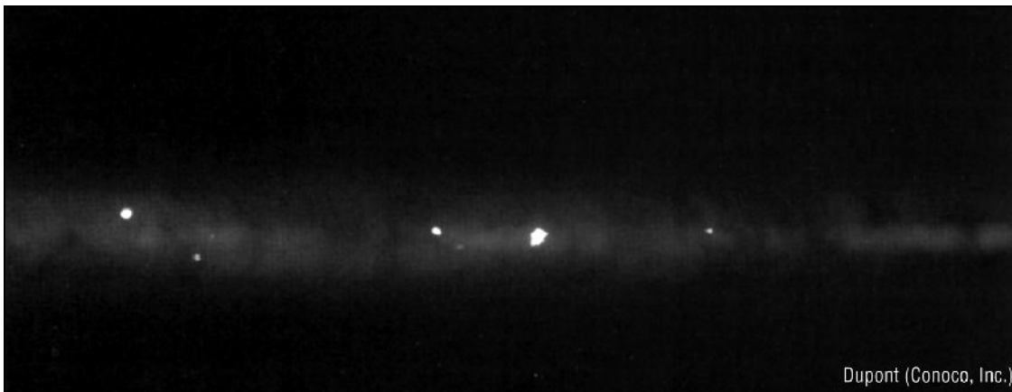
Figure 9.22—Radiographic Image of Tungsten Inclusions
