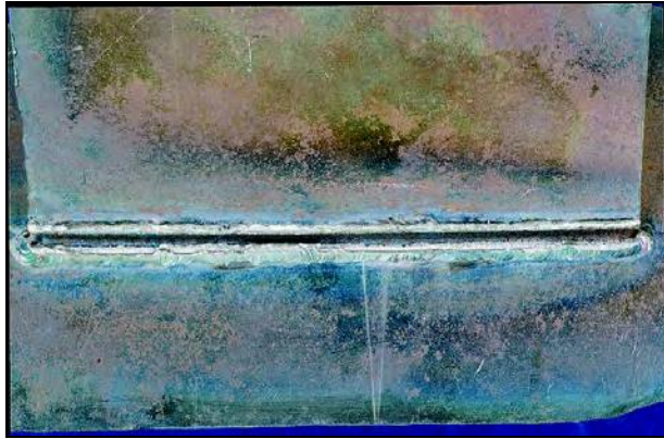
Figure 6.30—Fillet Weld Break Specimen
