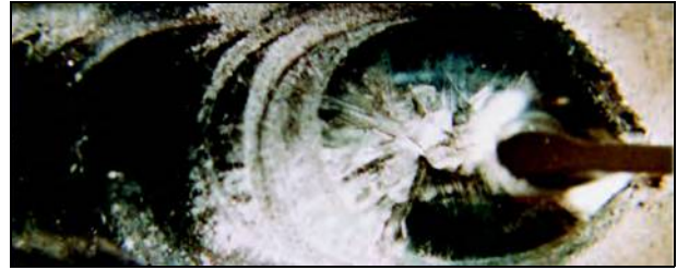
Figure 9.6—Closeup of Crater Cracks in Aluminum Weld
