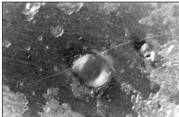
Figure 9.42—Crack Formed at Weld Spatter on Base Metal Surface
