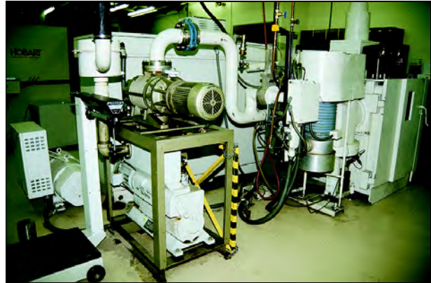
Figure 3.46—Exterior View of an Electron Beam Vacuum Pump
