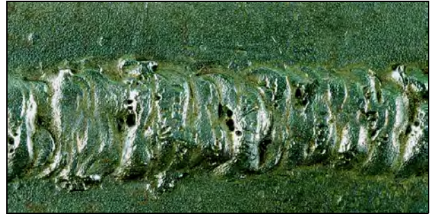
Figure 9.25—Isolated Surface Porosity
