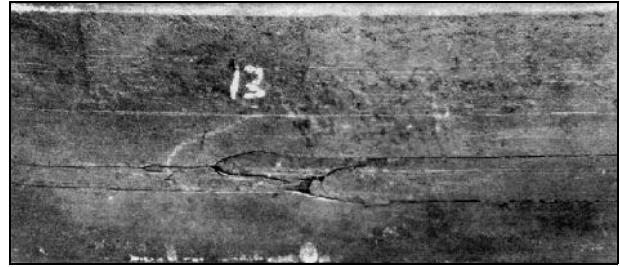
Figure 9.46—Deep Seam on the Surface of a Semi-Finished Rolled Product
