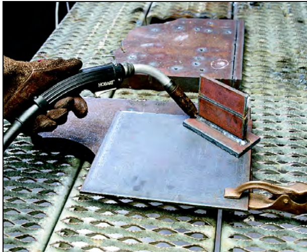
Figure 3.9—Gas Metal Arc Welding, Including Schematic of Details
