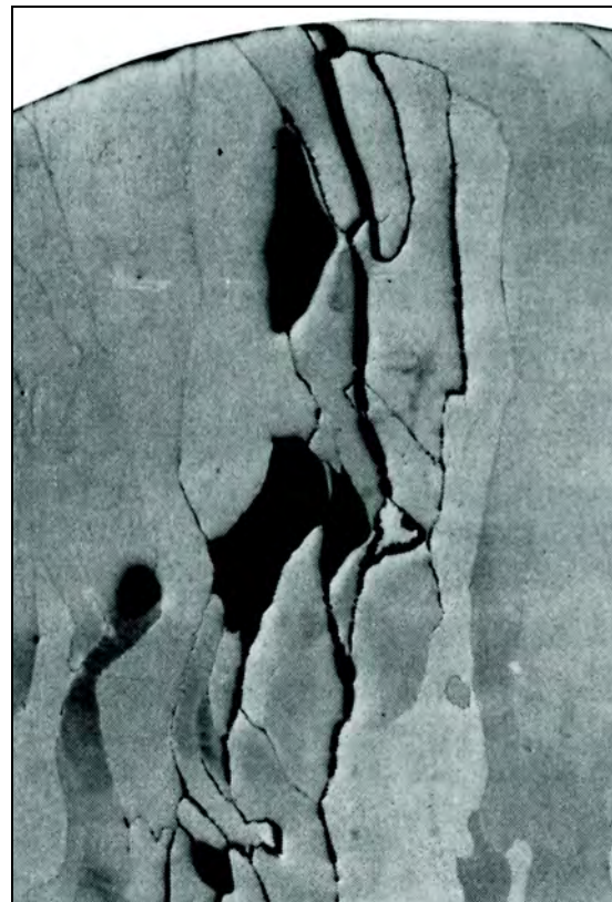
(C) Intergranular Corrosion in a Ferritic Stainless Steel GTA Weld
