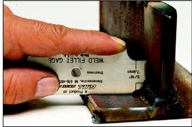
Figure 10.13—Use of Template Type Fillet Gauge
