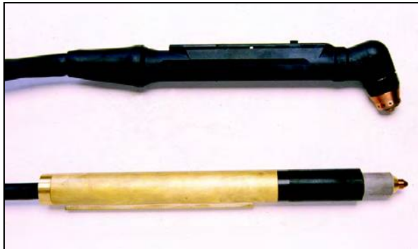
Figure 3.66—Typical Manual and Machine Plasma Arc Cutting Torches
