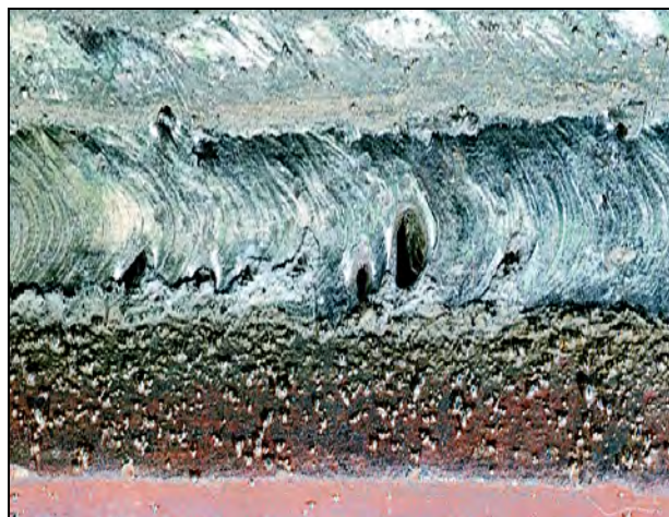
Figure 9.43—Weld Spatter on Base Metal
