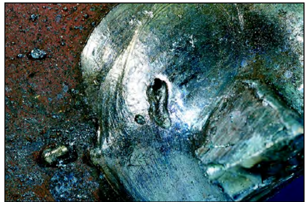
Figure 9.26—Elongated Surface Porosity
