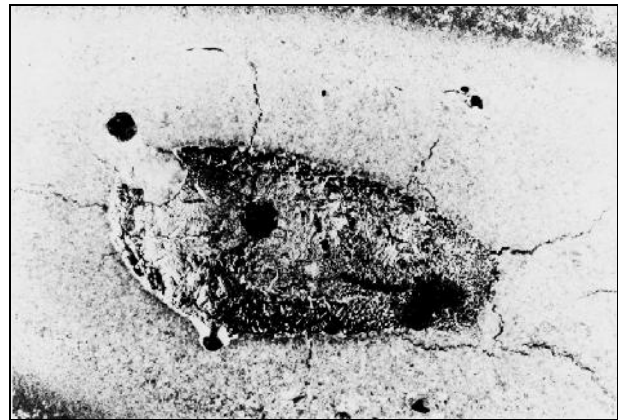
Figure 9.41—Photomicrograph of Martensitic Structure Produced by an Arc Strike
