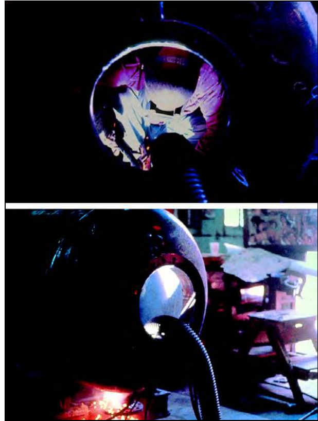
Figure 2.9—Welding in Confined Spaces
