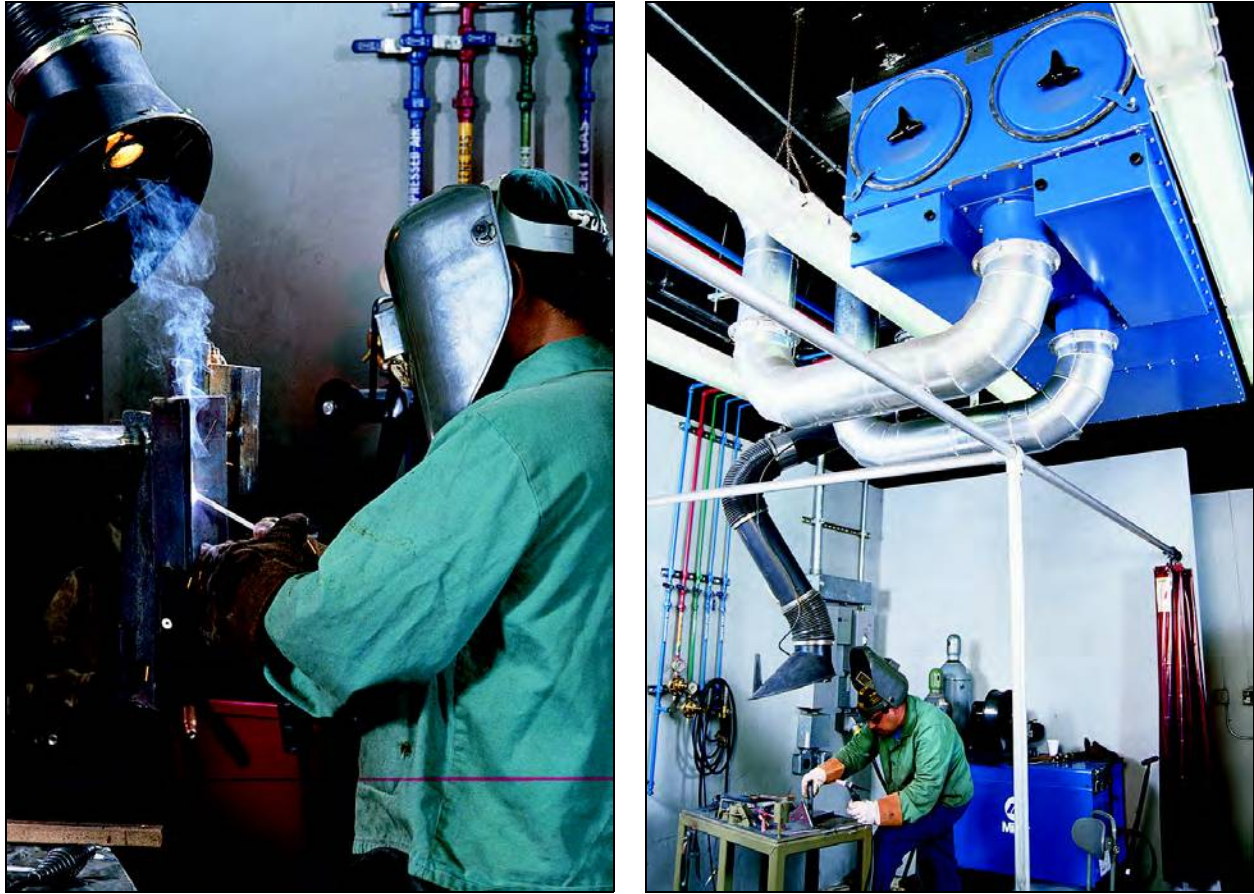
Figure 2.8—Movable Fume Extractor Positioned Near the Welding Arc
