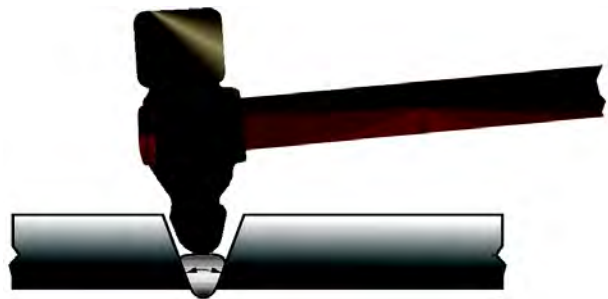
Figure 8.17—Peening of Intermediate Weld Layers to Relieve Welding Residual Stresses
