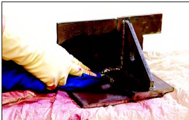
Figure 10.17—Excess Penetrant Removed
