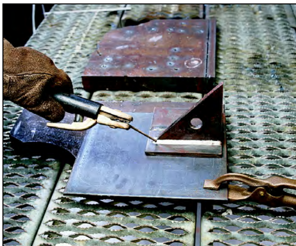
Figure 3.2—Shielded Metal Arc Welding, Including Schematic of Details
