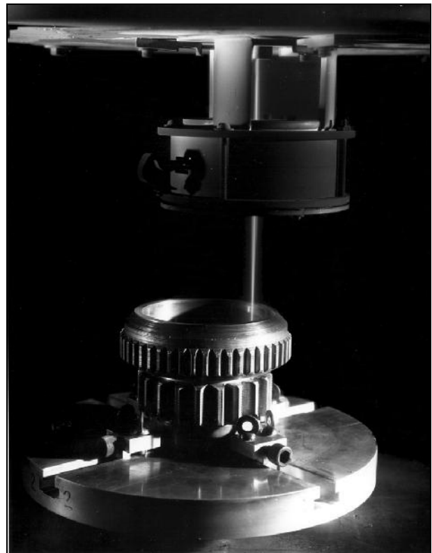
Figure 3.50—Electron Beam Welding a Gear in Medium Vacuum
