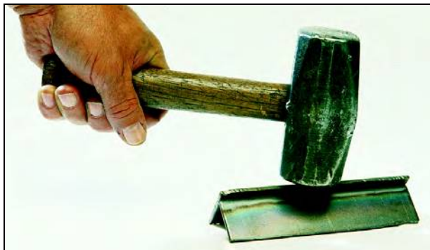
Figure 6.31—Method of Rupturing Fillet Break Specimen
