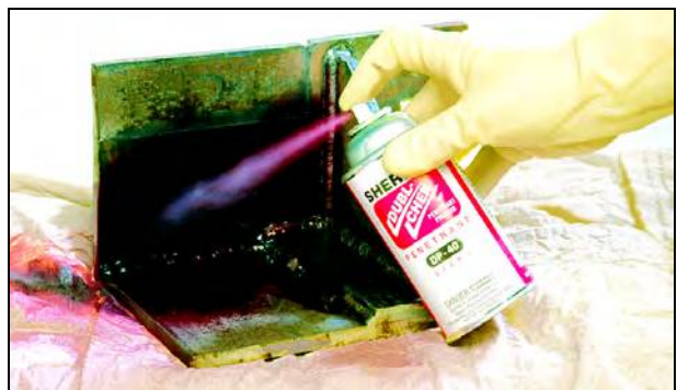
Figure 10.16—Penetrant on Test Surface and In Crack
