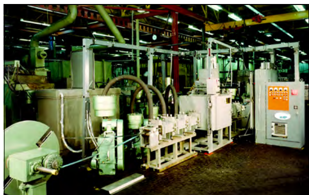
Figure 3.48—Electron Beam Welding Machine Designed for Joining Bimetallic Strip
